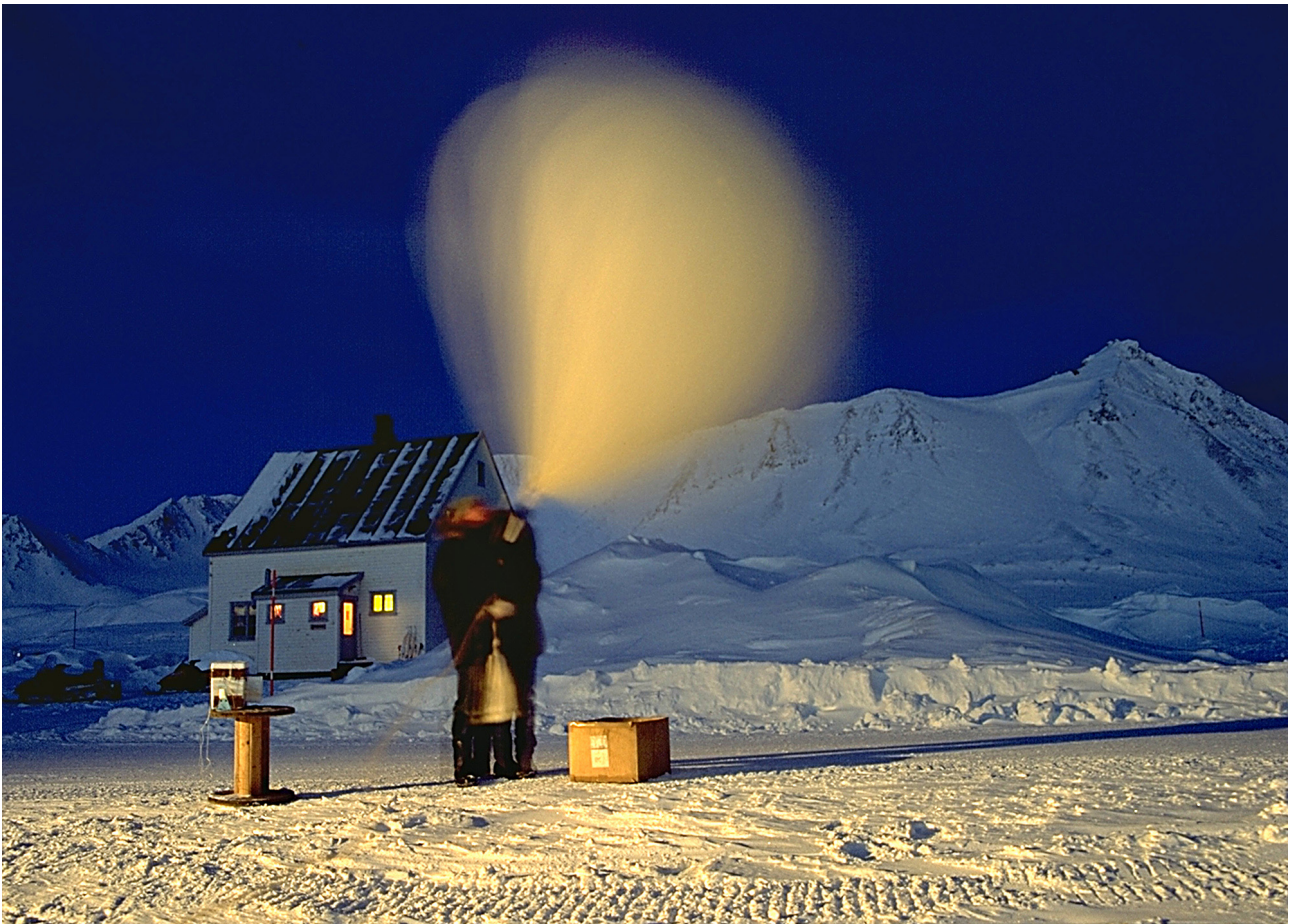
An ozonesonde is launched from Ny-Ålesund, Spitzbergen, in order to watch the state of the ozone layer in the Arctic. Photo: Thomas Seiler; Alfred Wegener Institute for Polar and Marine Research.
