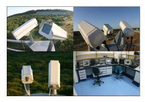
**Figure 1.** Images of the control room and some of the high sensitivity CCD video cameras of the CIECEM meteor observing station.
