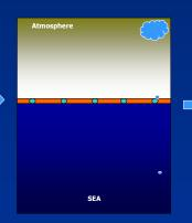
SAAs tend to gather at the free surface; such process is called adsorption. The presence of SAAs at the water surface reduces the surface tension, which in turn reduses the surface energy.
