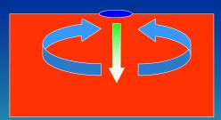
Mechanism of the gravity convection caused by the density excess at the free surface. SAAs play a secondary role.
