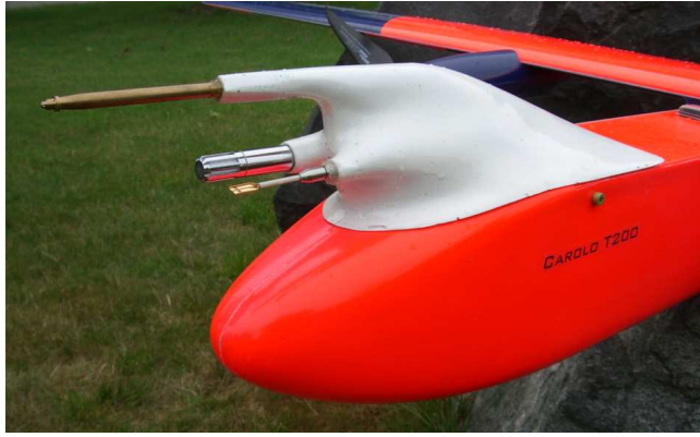
Figure 2: M^2AV meteorological measurement sensors.
